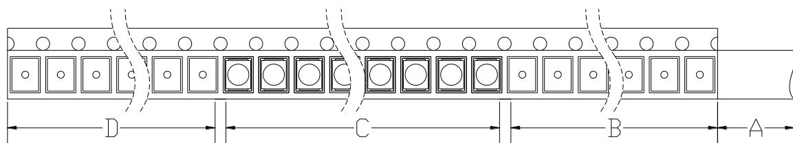
A: Top Cover Tape, 300mm; B: Leader, Empty, 200mm; C: 1000 Lamps Loaded; D: Trailer, Empty, 200mm.
